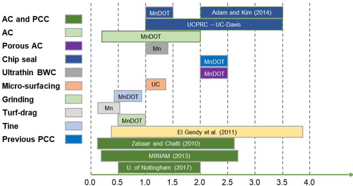
Figure 3-3 MPD ranges for various pavement surface types.
