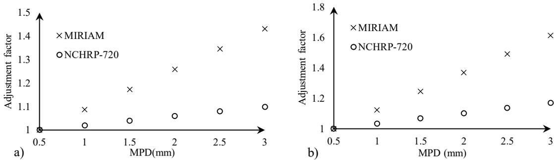
**Figure 2-3 Comparison of RR models, specifically the NCHRP 720 report and the MIRIAM project for a (a) car and (b) a heavy truck with trailer.**
