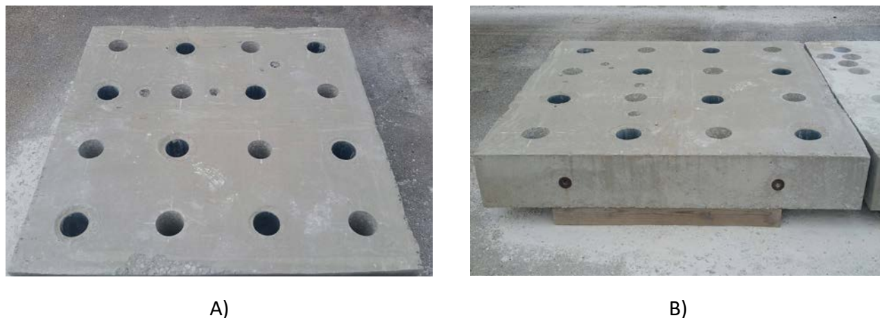
Figure 2.4. PCC Slabs for extracting the cores at the Illinois Center for Transportation (ICT).
