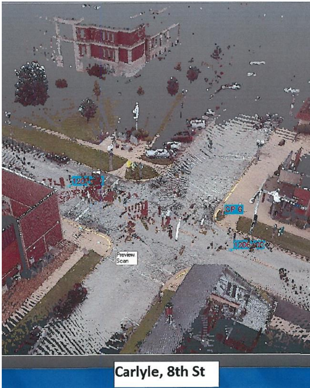
Figure 2: Contract No. 76H11, ADA ramps on US 50, 8th Street intersection generated from laser scanner point cloud with image superimposed.
