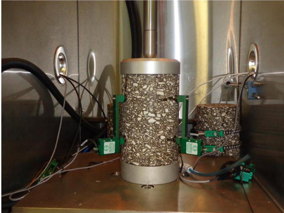
**Figure 21. Complex modulus test specimen and fixture with axial extensometers mounted to measure deformations.**
