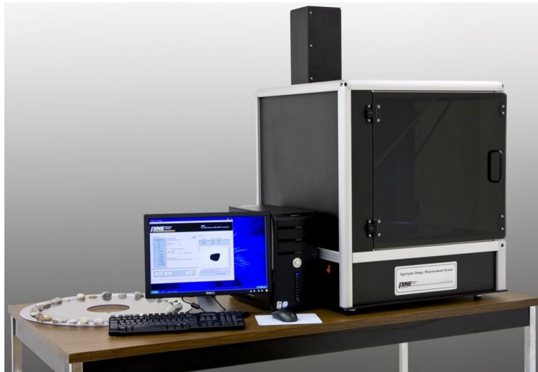
Figure 1.1 Second-generation Aggregate Imaging Measurement System (AIMS-II).
