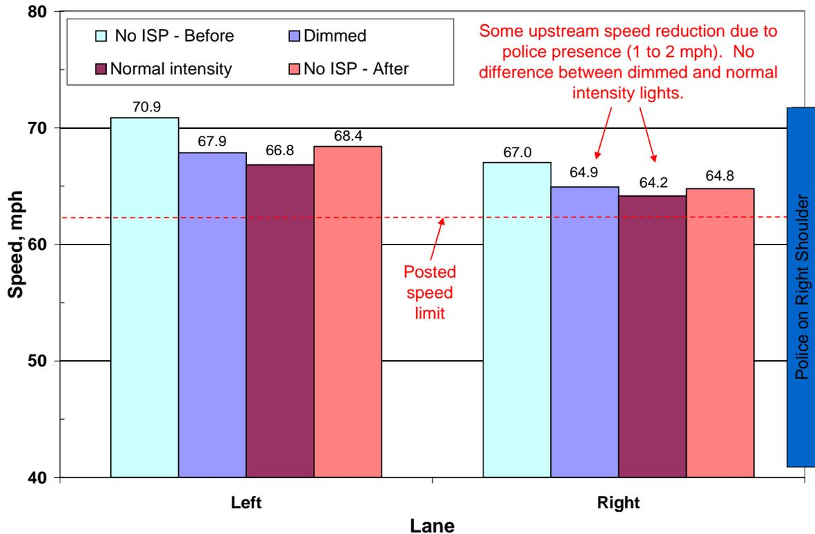
Figure 7.7 Upstream speeds—dimmed and normal-intensity lights.
