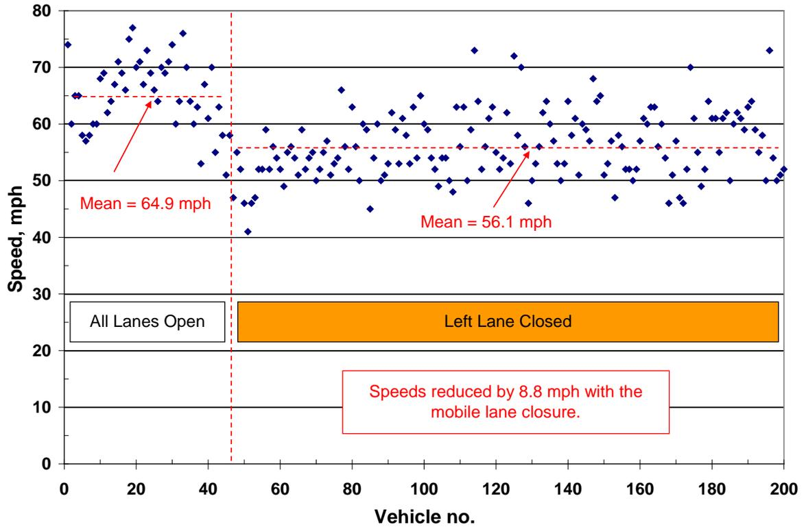
Figure 4.4 Speed data for the mobile lane closure on I-90 near the Des Plaines Oasis.
