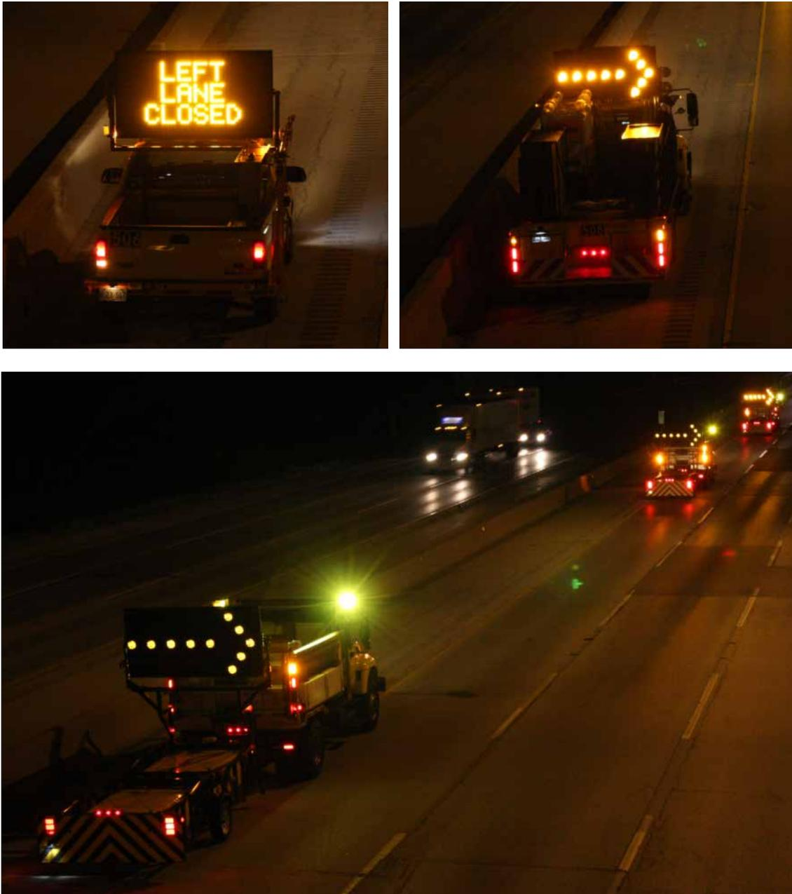
Figure 4.3 Vehicles and equipment used for the mobile lane closure on I-90 near the Des Plaines Oasis.
