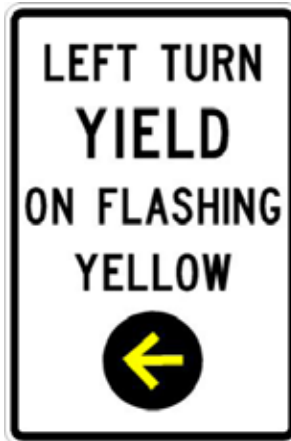
Figure 45. Supplemental signage installed at locations using the FYA indication (Source: Perez 2010).
