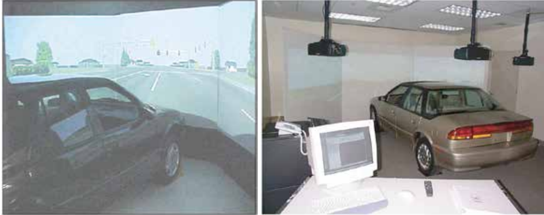
Figure 19. Typical driving simulators used in NCHRP 493 research (UMass on the left and TTI at Texas A&M on the right) (Source: Brehmer et al. 2003).
