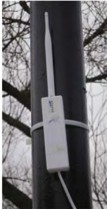
Figure1. Pole-mounted Wi-Fi monitor prototype. Wi-Fi monitors are based on low-cost, off-the shelf Wi-Fi base-station hardware, modified with custom traffic-monitoring firmware.
