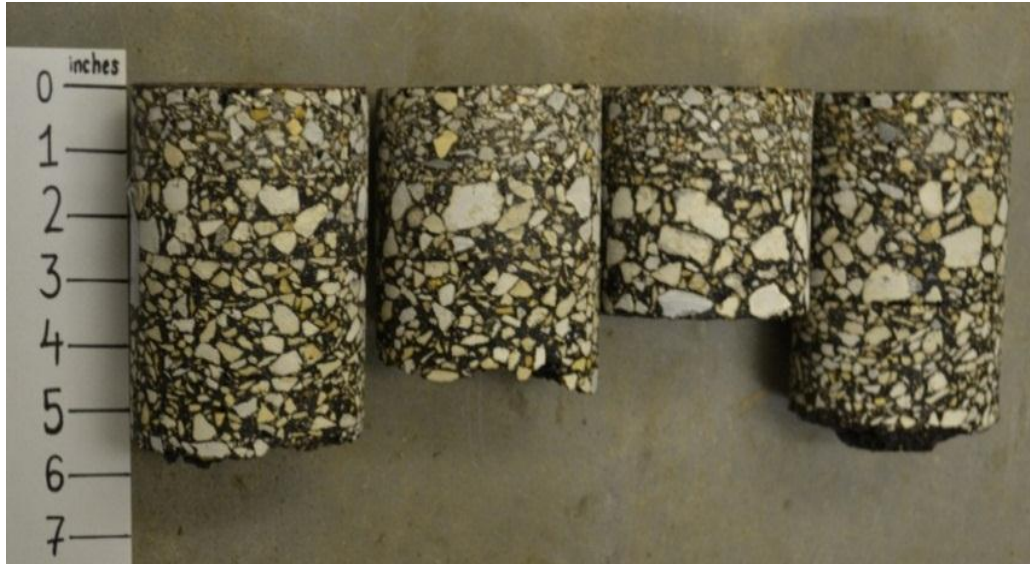
Figure 4.1. A sample of cored specimens from the IL-98 project.
