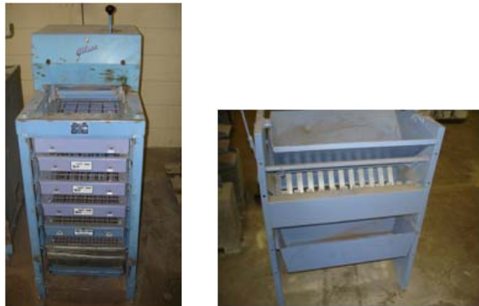
Figure 3. Photos showing the sieve shaker (right) and the sample splitter/mixer (left) at ATREL used in the experiment.
