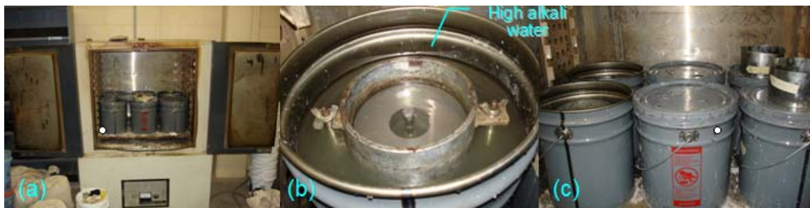
Figure 7. Storage of six specimens soaked in high alkali water in the oven at 70°C.
