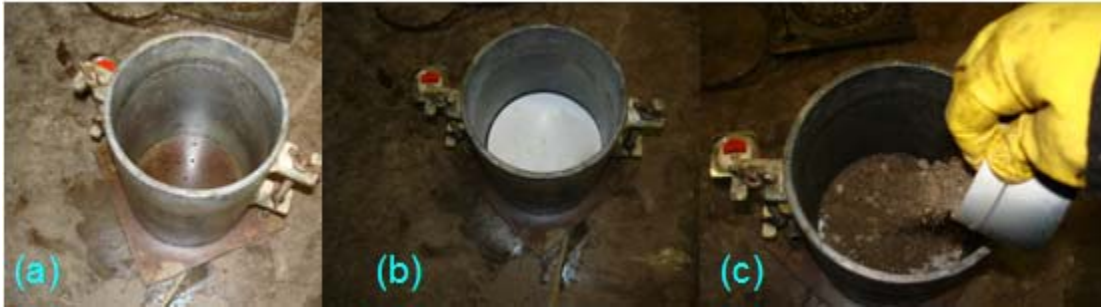
(a) coating with oil (The CBR molds were coated with a rust preventative - 10W motor oil - according to ASTM D 4792); (b) placing spacer disk over the base plate and then a filter paper on the disk; (c) placing material into the mold per layer;
