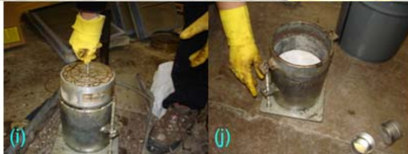
(f) trimming with a straightedge; (g) placing a filter paper on the top; (h) inverting the CBR mold; (i) removing spacer disk; (j) placing extension collar.
