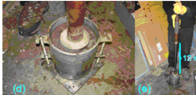
(d) & (e) materials prepared in CBR molds were compacted in three layers with 56 blows per layer by using a 10-lb rammer dropping from a height of 18 in.;
