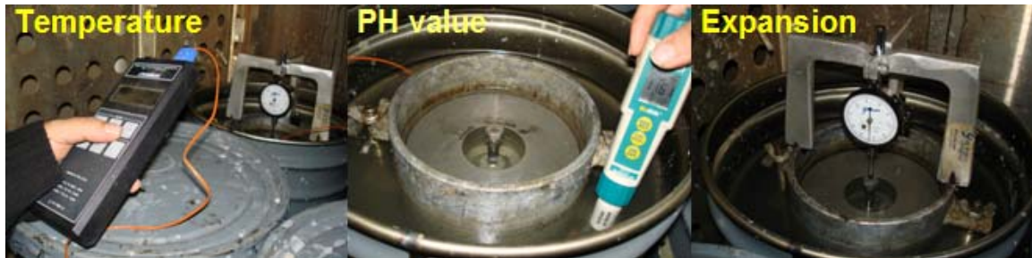
Figure 8. Photos describing continuous data collection of both temperature and pH values of the solution and the specimen expansion values during testing.
