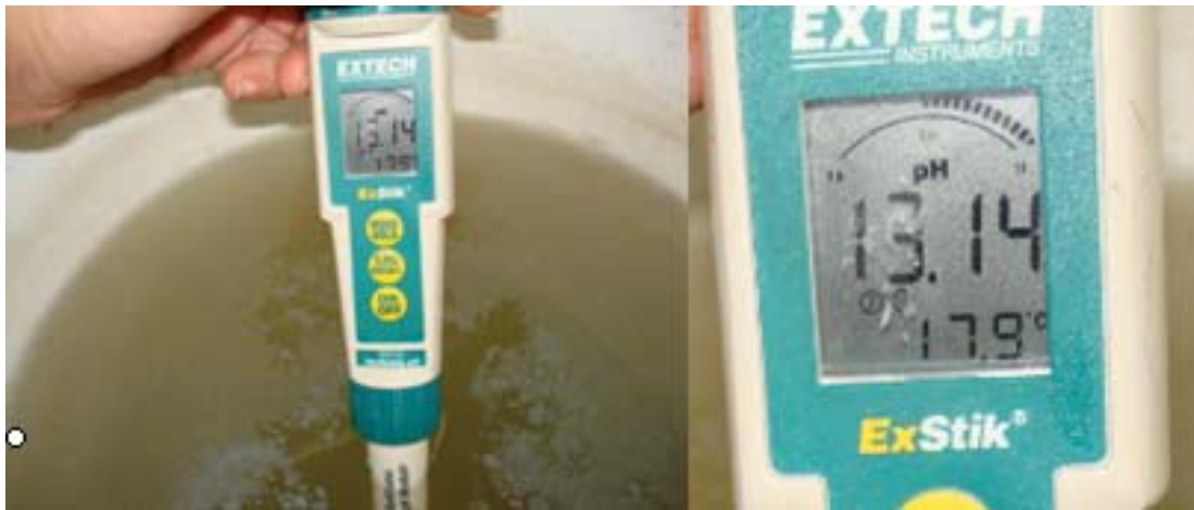
Figure 6. Measuring pH value of the high alkali solution at room temperature.
