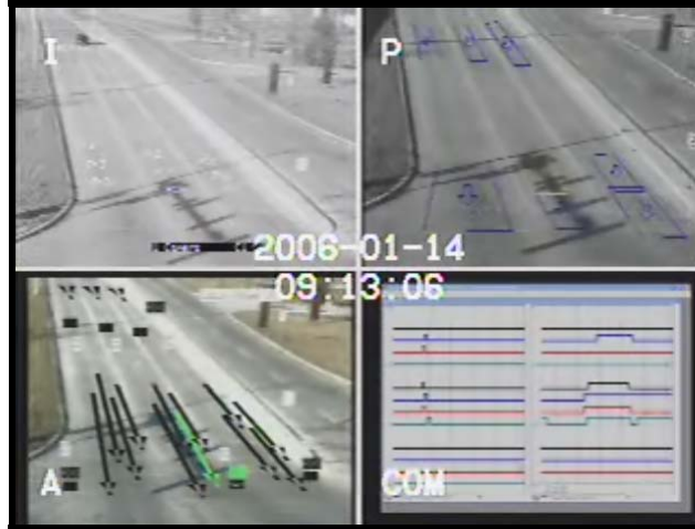
Figure 4.1. Sample image of stuck-on calls caused by shadow of mast arm from crossing street.
