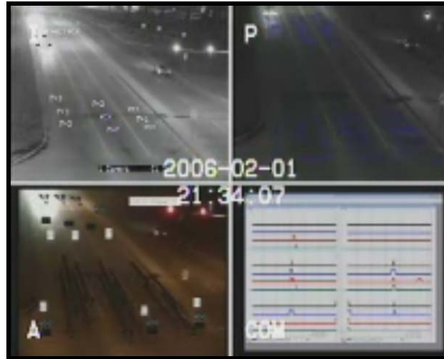
Figure 4.6. Sample of a missed vehicle due to bright vehicle headlights.
