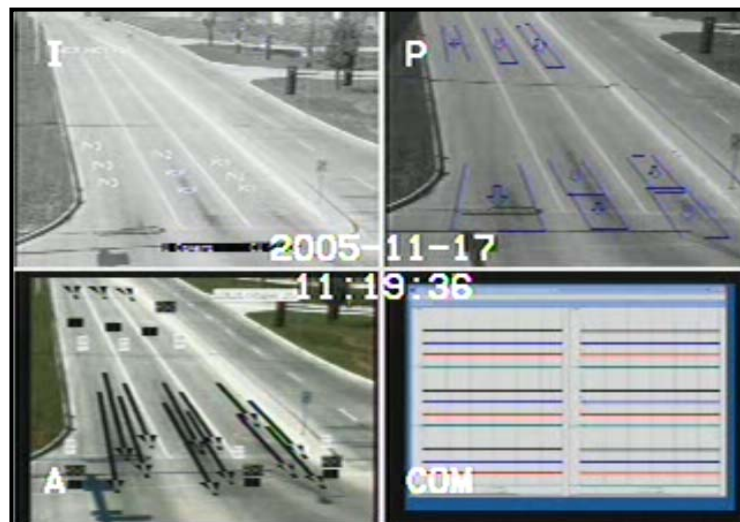
Figure 3-9. VD configuration in manufacturers' best setup (Setup 2).
