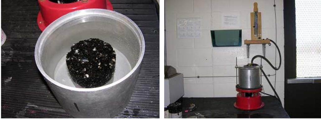
Figure 3-4. HMA-PCC specimen in vacuum container.
