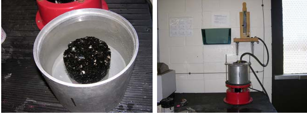
Figure 3-4. HMA-PCC specimen in vacuum container.
