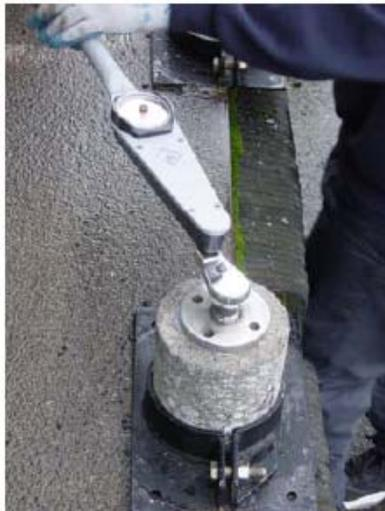
Figure 2-9. Torque bond test (Tashman et al. 2006).
