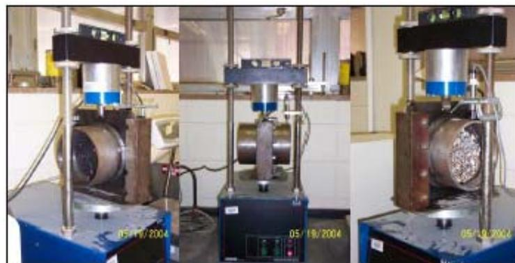
Figure 2-7. Laboratory bond interface strength device, LBISD (Woods, 2004).
