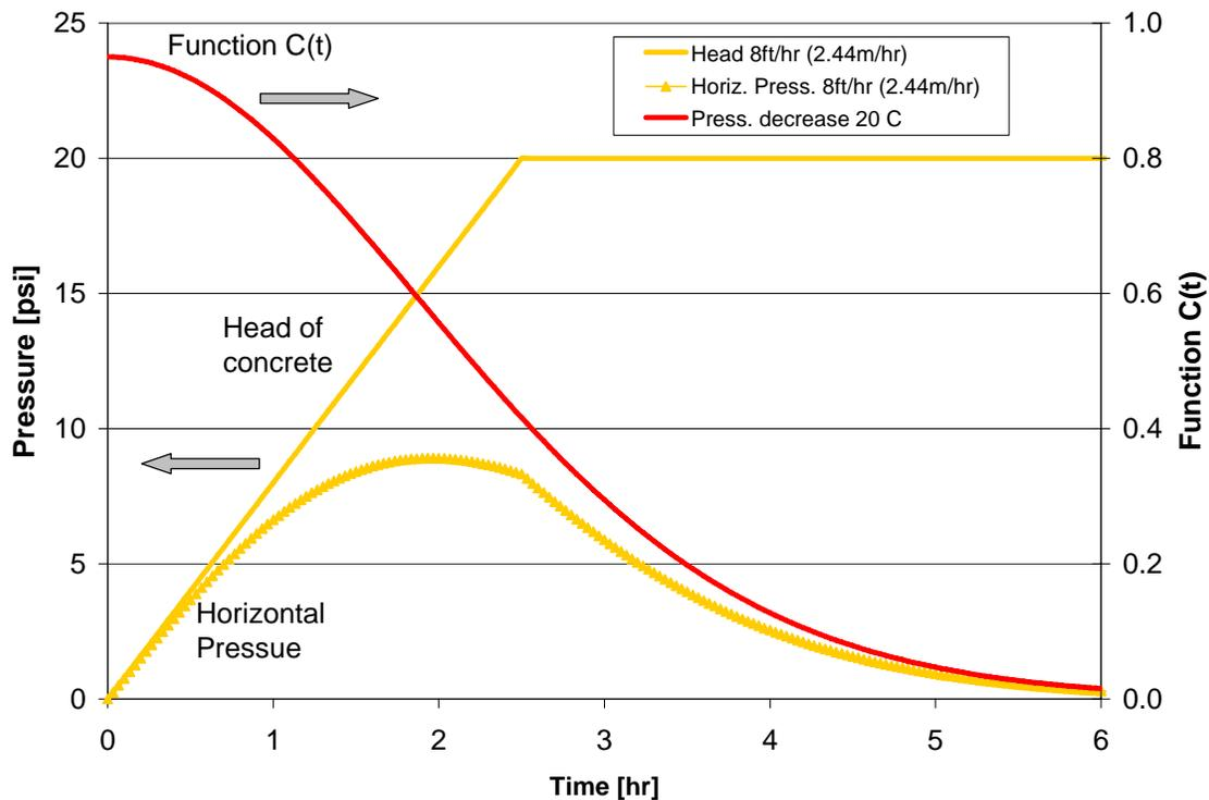
Figure 14. Model predicts horizontal formwork pressure for a given SCC with behavior described by  $C(t)$  while the pressure head increases as a function of concrete depth above the sensor location [4]. (1 psi = 7 kPa).
