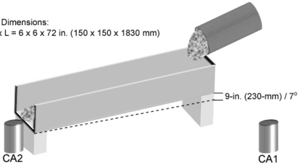
Figure 5. Flow trough for dynamic segregation [2].
