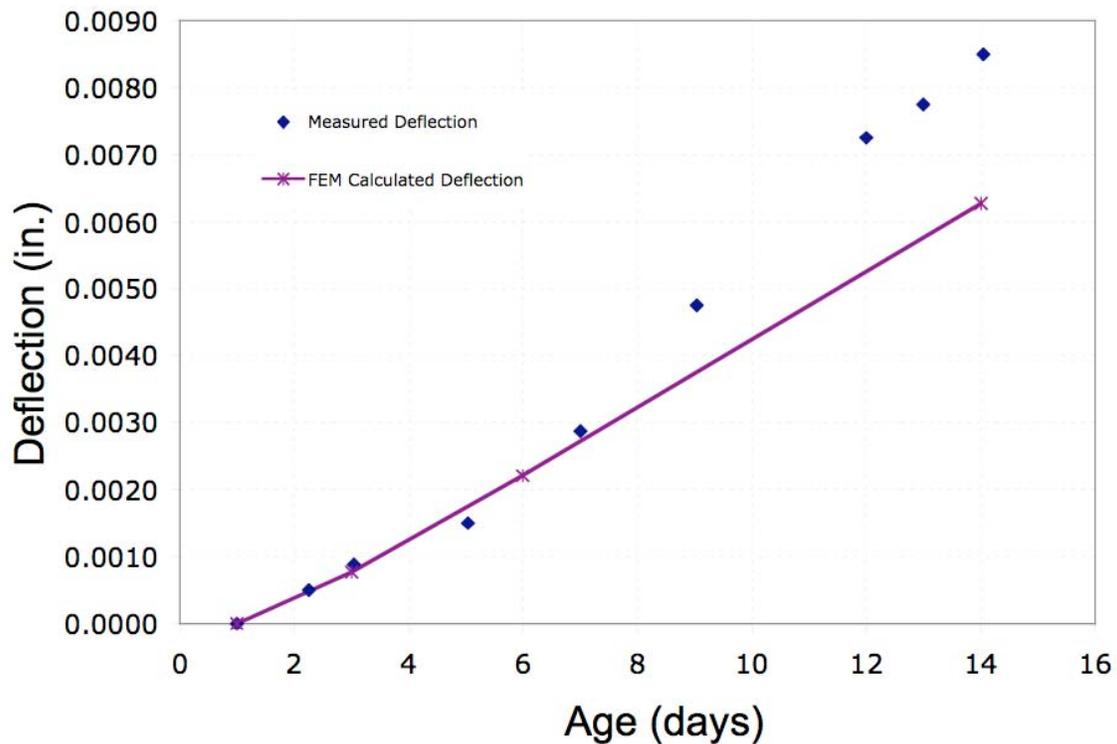
Figure 10. Calculated vs. measured cantilever deflection [2]. (1 in. = 25 mm\*).
