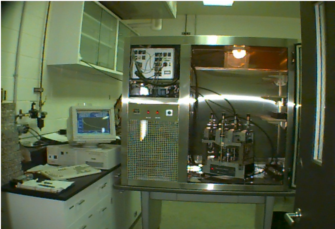
Figure 2. Beam fatigue equipment.
