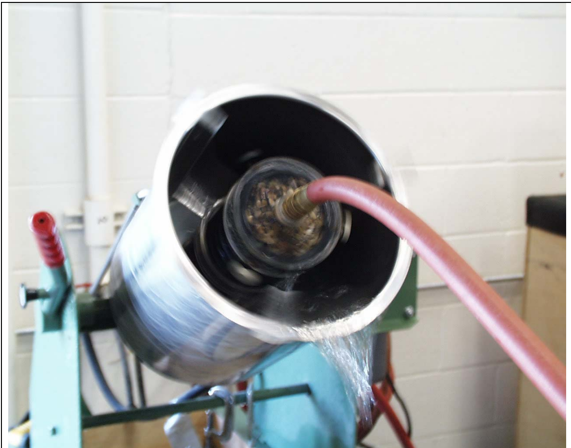
Figure10. Pipe Slot Infiltration Test in Progress at ATREL
