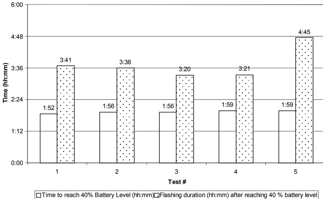
The estimate of the error from the true mean for time to reach 40% battery level is 1.94 minutes and for flashing duration after reaching 40 % battery level is 7.88 minutes (based on the first four observations only). These values correspond to 1.67 and 3.75 % of their means. Therefore further testing was not performed. The average time to reach 40% battery level is 1:56 and average flashing duration after reaching 40 % battery level is 3:30 (based on the first four observations only).
