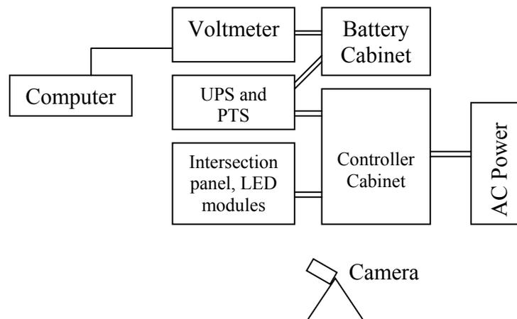
Figure 1. Block diagram of the experimental setup.
