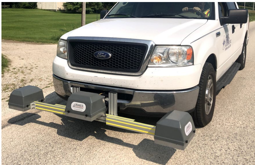
Figure 7. Photo. High-speed texture profiler used in field testing.
